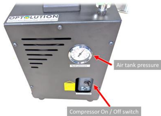
Figure 3: Compressor main power switch.
