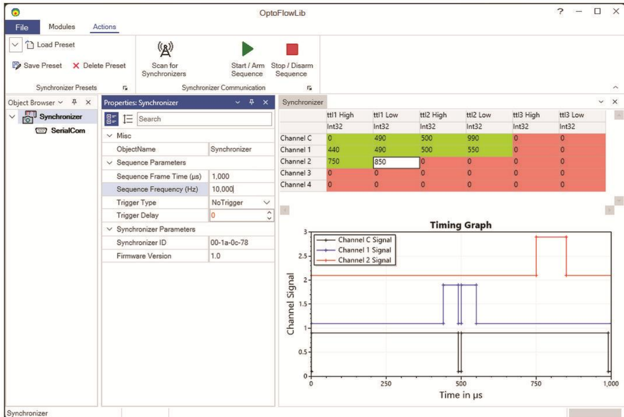
Figure 19: Screenshot of the oltSync software. This software can be used to configure the synchronizer for use with any Laser or camera, and without PIVlab. The timing sequence for all five channels can be set as needed.
