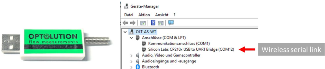
Figure 15: Left: The wireless USB dongle. Right: Verification of driver installation in Windows device manager.
