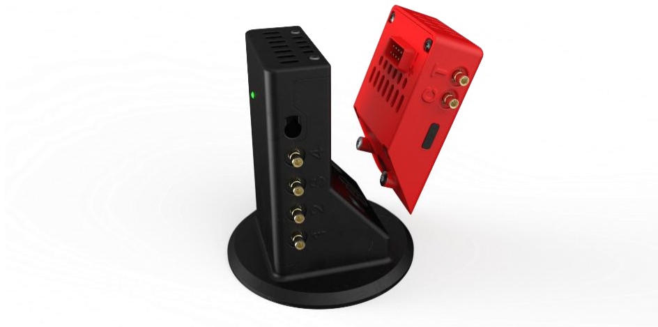
Figure 5: When the synchronizer is used as stand-alone device, it is attached to the Synchronizer Dock.
