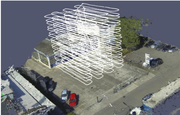
Flight path of the OPTOkopter: The surrounding area is mapped in 3D during or before the wind measurement.
