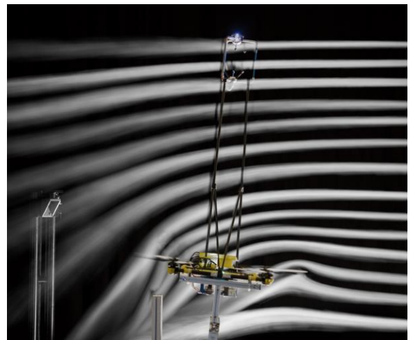
Stream lines in the wind tunnel (5 m/s).
