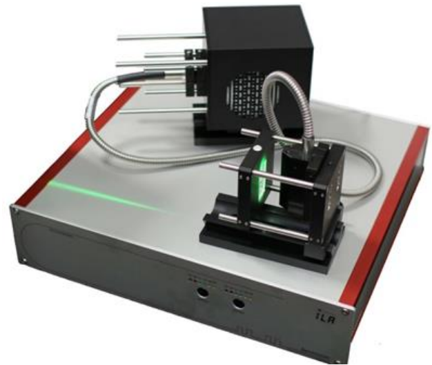
Fig. 4: LED-Head with fiber optic light sheet (FLOS) on Synchronizer
