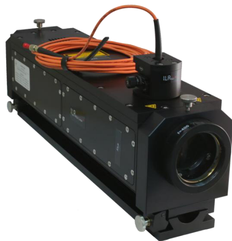
Fig.2: 2D fp50-shift probe detached from combined probe
